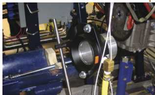
A Model 120024 4" (102mm) Super Air Amplifier cools an engine during dynamometer testing.
