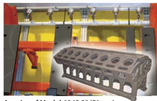
A series of Model 6042 2" (51mm) Adjustable Air Amplifiers blow coolant off 16 cylinder diesel engines.
