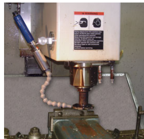
The Adjustable Spot Cooler replaces flood coolant and eliminates hours of cleanup on a cast iron machining operation.
