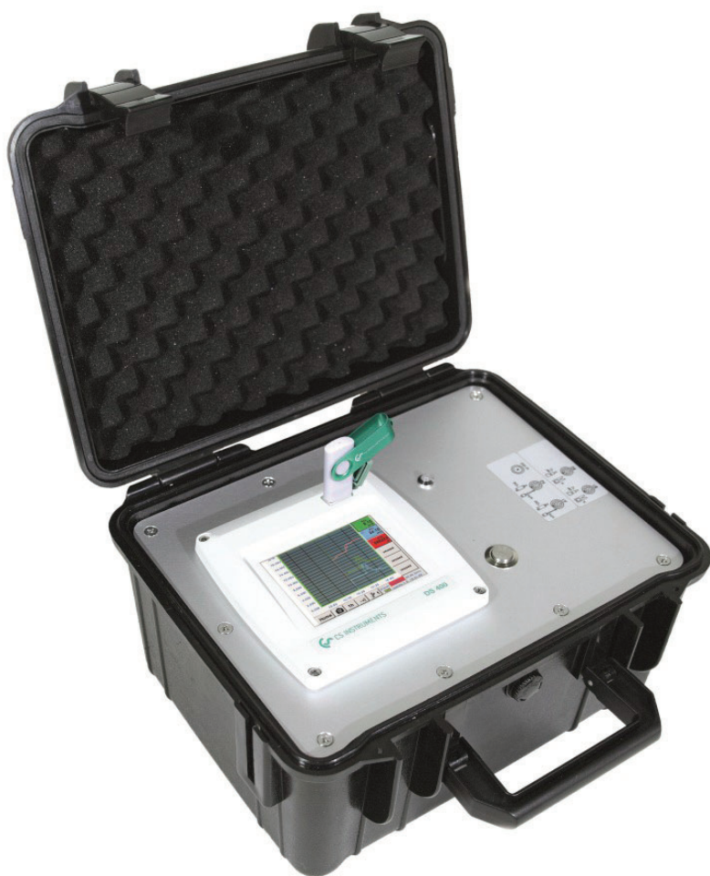
Up to 4 sensors can be connected including power supply for all sensors
