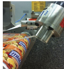
1" (25mm) Line Vac remove and discard a label matrix.
