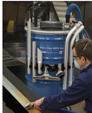
A technician uses a Heavy Duty HEPA Vac to perform scheduled maintenance on a pulverizer.
