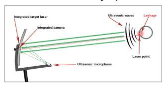
By focusing the ultrasonic waves in the parabolic mirror, even the smallest leaks of 0.8 l/min (approx. € 8 p.a.) can be located with pinpoint precision (± 15 cm) at a distance of up to 10 to 15 m.
