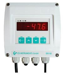
The DS 52 has 2 potential-free alarm contacts (changeover contacts) which can be charged with a maximum of 230 VAC, 3 A. The alarm thresholds are freely adjustable with the keys.
