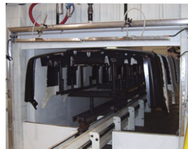
Bumpers, car bodies and fascia are cleaned of dust and fibers prior to painting.
