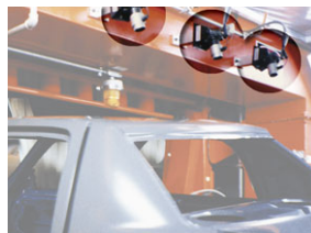
(3) Ion Air Cannons blow contaminants from car bodies prior to painting.
