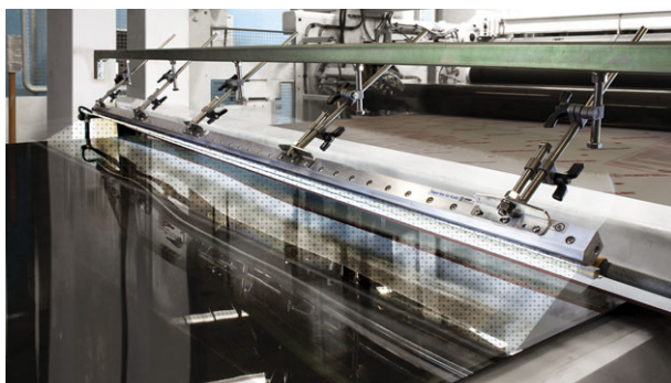
This 96" Long Super Ion Air Knife cleans an acrylic sheet before protective wrap is applied.
