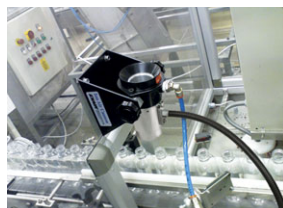
The Model 8292 Ion Air Cannon System eliminates the static and dust prior to filling the bottles.
