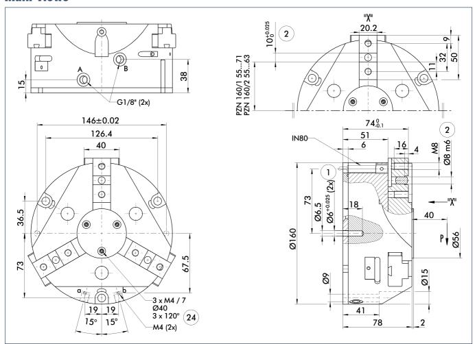
The illustration shows the gripper in the basic version with closed jaws, without taking into account the measurements of the optional extras described below.
