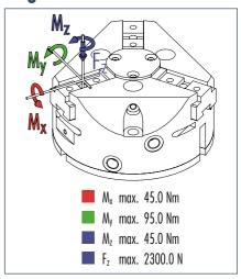
① Moments and forces apply per base jaw and may occur simultaneously. M<sub>V</sub> may arise in addition to the moment generated by the gripping force itself. If the max. permitted finger weight is exceeded, it is imperative to throttle the air pressure so that the jaw movement occurs without any hitting or bouncing. The tool life may be reduced.
