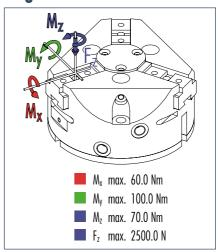
Moments and forces apply per base jaw and may occur simultaneously. My may arise in addition to the moment generated by the gripping force itself. If the max. permitted finger weight is exceeded, it is imperative to throttle the air pressure so that the jaw movement occurs without any hitting or bouncing. The tool life may be reduced.
