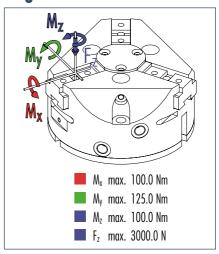
Moments and forces apply per base jaw and may occur simultaneously. M<sub>V</sub> may arise in addition to the moment generated by the gripping force itself. If the max. permitted finger weight is exceeded, it is imperative to throttle the air pressure so that the jaw movement occurs without any hitting or bouncing. The tool life may be reduced.
