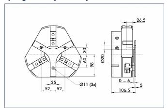
For spring-mounted positioning of the workpiece against the stop after the gripper has opened. Developed especially for the loading of machining centers.
