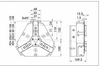
The "Dust-proof" option increases the degree of protection against penetrating substances. The screw connection diagram moves by the height of the intermediate jaw. The finger length must still be measured from the upper edge of the gripper housing.
