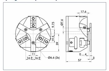
For spring-mounted positioning of the workpiece against the stop after the gripper has opened. Developed especially for the loading of machining centers.
