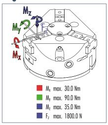
1 Moments and forces apply per base jaw and may occur simultaneously.  $M_{V}$  may arise in addition to the moment generated by the gripping force itself. If the max. permitted finger weight is exceeded, it is imperative to throttle the air pressure so that the jaw movement occurs without any hitting or bouncing. The tool life may be reduced
