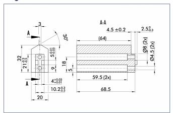
Finger blanks for customer-specific reworking, incl. screw connection diagram
