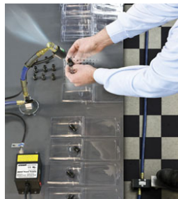
The Gen4 Model 8910 Instant Static Elimination Station removes contaminants on plastic fittings prior to packaging.
