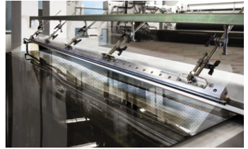
This 96" Long Gen4 Super Ion Air Knife cleans an acrylic sheet before protective wrap is applied.
