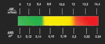
A typical specific power of an oil-injected compressor can be as follows:
