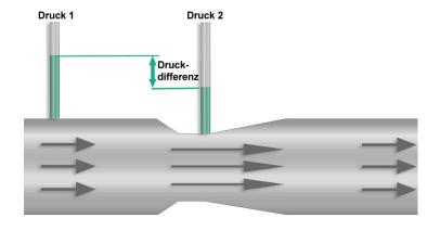
For differential pressure measurement, two separate lines lead to a differential pressure measuring cell. One pressure connection (pressure 1) is located at the inlet of the Venturi tube and a second pressure connection is located at the outlet of the Venturi tube (pressure 2). Without flow, the pressure at the inlet and outlet is identical.
