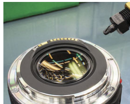
This PEEK material Atto Super Air Nozzle was chosen because of its non-marring quality for a blow off application on a sensitive lens.
