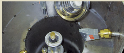
2" Flat Super Air Nozzles blow off metal parts as they are lifted through a vacuum chamber.
