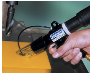
Model 6394 Deep Hole Vac-u-Gun All Purpose System removes the chips from a drilled plastic part.
