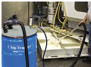
The Chip Trapper pumps the coolant back into the sump - free of chips and debris.
