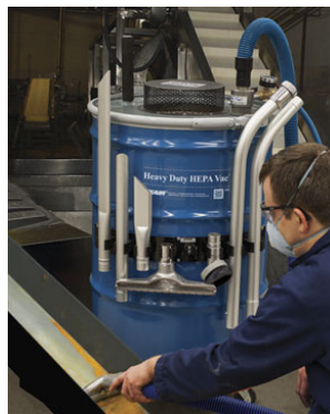
A technician uses a Heavy Duty HEPA Vac to perform scheduled maintenance on a pulverizer.
