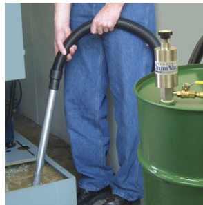
Reversible Drum Vacs are designed to fit the 3/4 NPT bung of any closed top drum. This model 6196-30 30 gallon system empties the coolant sump of a CNC.
