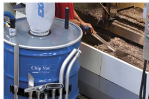
110 Gallon Chip Vac offers maximum capacity cleanup on a large machining operation.
