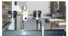
(2) Model 120022 2" (51mm) Super Air Amplifiers dry small parts as they move down along a parts conveyor.
