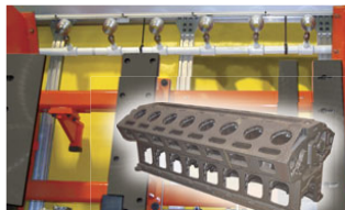
A series of Model 6042 2" (51mm) Adjustable Air Amplifiers blow coolant off 16 cylinder diesel engines.
