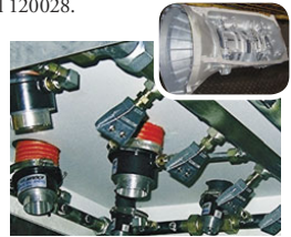
Model 120022 2" (51mm) Super Air Amplifiers and Model 1122 2" Flat Super Air Nozzles blow off transmissions after they are machined.
