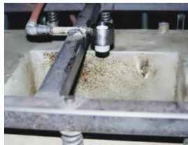
A Model 121021 1-1/4" (32mm) High Temperature Air Amplifier directs hot air to a rotational mold cavity for uniform wall thickness of the plastic part.
