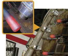
Model 6042 2" (51mm) Adjustable Air Amplifiers with swivel fittings cool inductively heated axes prior to installing the hubs.
