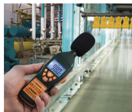
The Sound Level Meter identifies a potential source of hearing loss.
